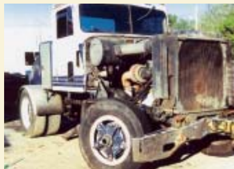
Right front quarter view of truck shows the hood, grille and fenders, which were torn off in the accident.
